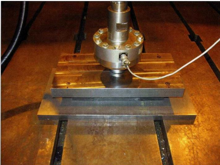
Figure 2: Compression test set-up – Load cell, support and loading fixtures
