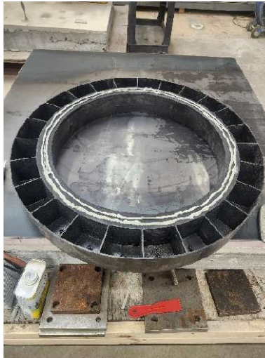
Figure 2.2: The bottom of the 4-inch ring with the lip removed and sealant applied
