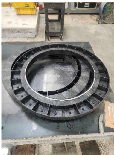
Figure 2.3: 2-inch riser ring with sealant
