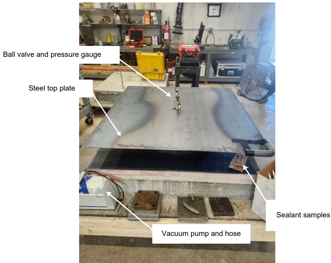
Figure 2.4: Riser ring assembly
