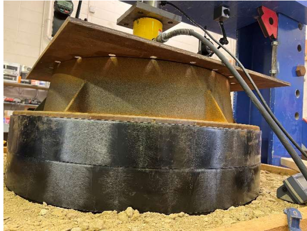
Figure 2.2: Riser rings on compacted Class 5 and cast-iron frame and cover
