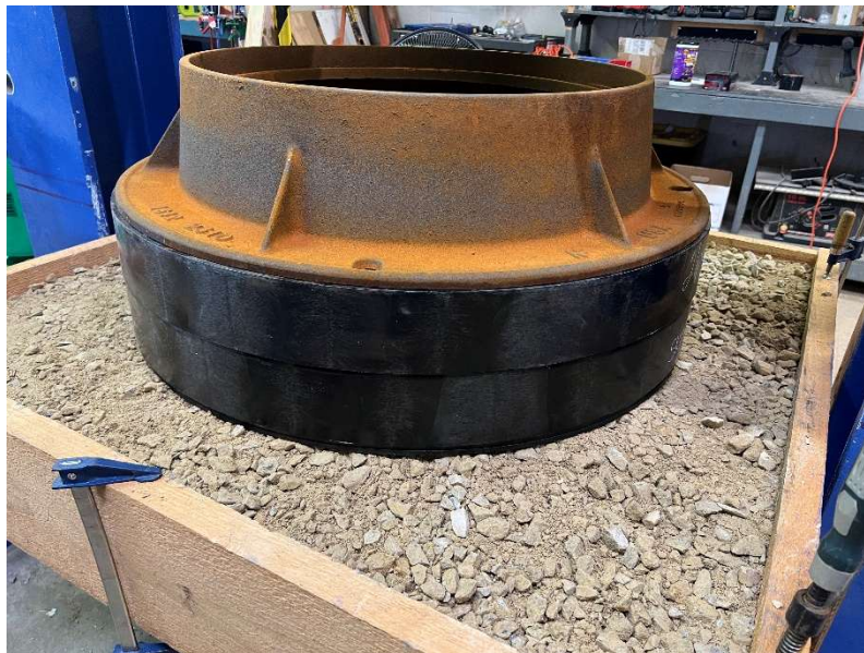
Figure 2.1: HDPE riser rings and casting on top of Class 5 Material
