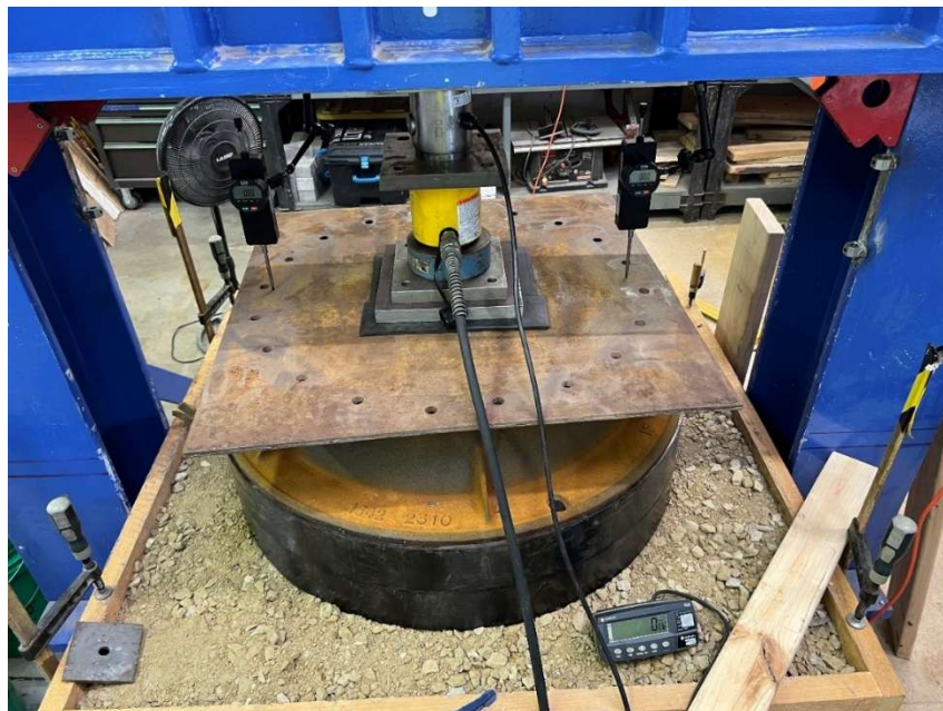
Figure 2.3: Riser ring assembly surrounded by load frame, bearing plate, load cell, spacer, deflection gauges, load-cell monitor, and hydraulic jack
