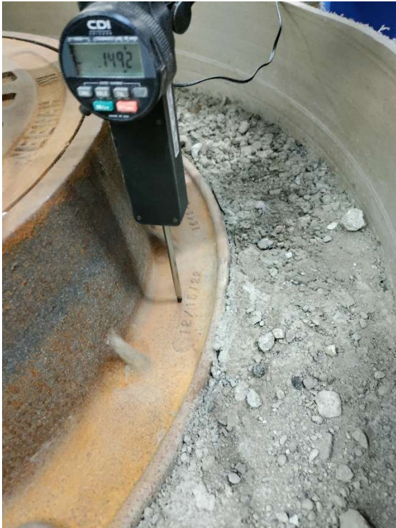
Figure 2.5: Deflection gauge contact – North
