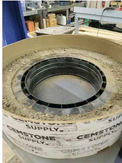
Figure 2.2: Compacted Class 5 flush with the top of the HDPE risers
